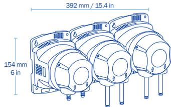
Pump 1 is set as pH by default. All pumps can be set as pH or nutrient in Bluelab Connect.
