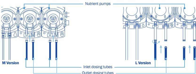
**Note:** If pH adjuster or nutrient stock solution being used has solid particles suspended in it, then a sieve filter should be placed on the end of the tube to prevent tube blockages and potential damage to the peristaltic pumps.
